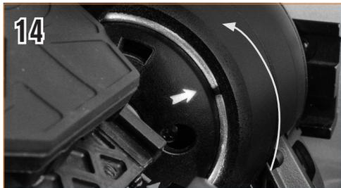
Line up the arrow on the dock with the alignment mark on the mount and press inward while turning the dock counterclockwise until the orange release button snaps into place in the hole on the dock.
