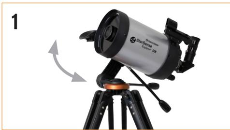
The StarSense Explorer DX mount has slip clutches in both axes. To make large movements with the telescope, simply hold a tripod leg with one hand and use the other hand on the telescope tube to push the telescope in the desired direction.
