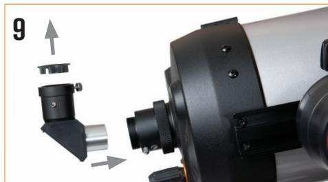
9 Locate the erect image diagonal and remove the plastic covers. Insert the barrel of the diagonal into the back of the telescope tube and secure in place by tightening the set screws.
