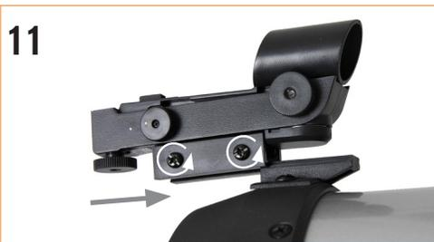
Loosen the two Phillips head screws on the side of the finderscope and slide the finderscope onto the mounting dovetail on the top of the telescope tube. The large window on the finder should be facing the front of the telescope. Secure the bracket by tightening the Phillips head screws on the side of the finderscope.
