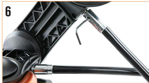
6 Place the slow-motion control knob over the D-shaped gear shaft and push inward to make sure it is fully seated. Use the hex key to tighten the setscrews onto the gear shaft. Return the hex key to its storage position in the front of the mount.
