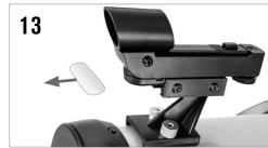
There is a small clear plastic tab inserted between the battery and the contact. This was included to prevent the battery from discharging during shipment. Pull this out to allow your battery to work.
