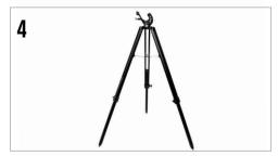
Check to ensure that all three legs are the same height once extended to provide a level platform for the telescope.
