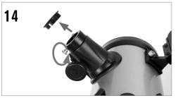
Loosen the setscrews on the telescope focuser and remove the dust cap.
