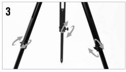
Extend the center portion of each of the three tripod legs down about 6 to 12 inches. Use the tightening screw on each leg to secure the extended leg in
