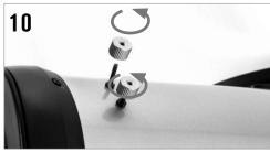
To install the finderscope, remove the two silver nuts from the threaded posts on the top of the tube, near the focuser.
