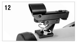
Thread the two nuts back onto the threaded posts.
