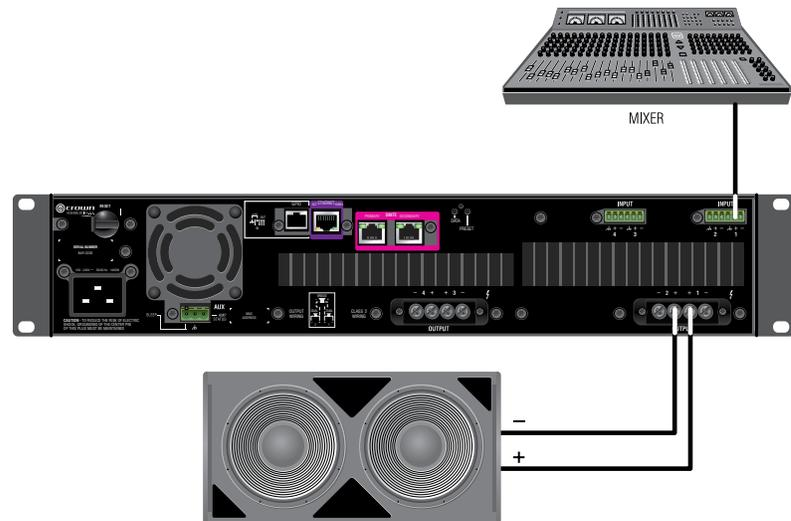
**Figure 9:** System wiring in bridge mono mode
