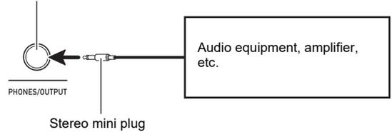
**■ Sounding Input From an External Device on the Digital Keyboard**
