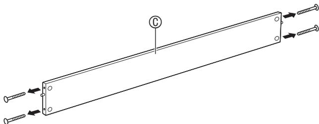
2. Attach side panels A and B to back board ©. Secure side panels A and B to the back board © using the screws you removed in step 1.
