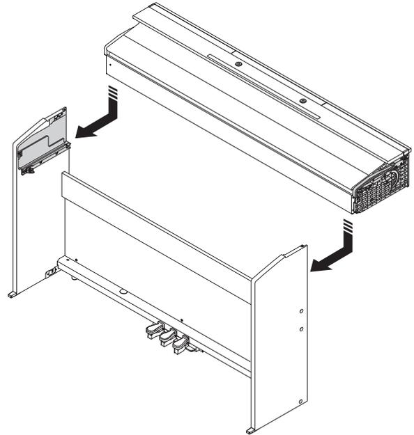
**10.** Use ⑯ screws to secure the piano to the stand from both the front and the back.
