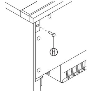
11. After checking to make sure the six screws that secure side panels **A** and **B** are fully tightened, cover the heads of the screws with screw caps **K**.
