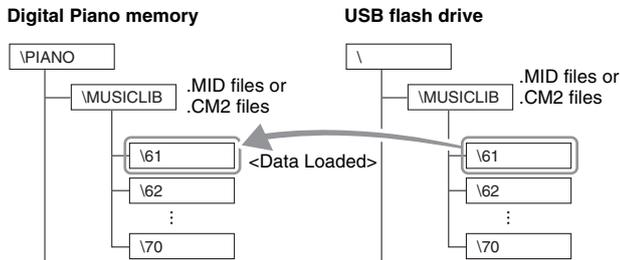
1. On your computer, copy the file you want to load to one of the numbered sub-folders (61 through 70) inside the "MUSICLIB" folder on the USB flash drive.
