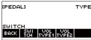
(2) Press VOL TYPE1 or VOL TYPE2 according to the polarity of the volume pedal.
