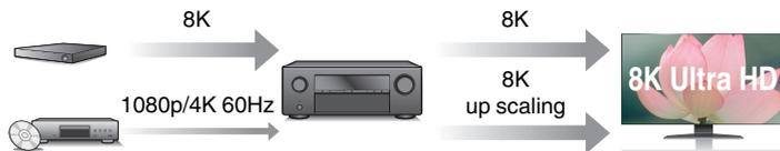
This unit is equipped with a 8K video upscaling function that allows 1080p/4K video to be output via HDMI at 8K (7680 × 4320 pixels) resolution. This function enables the device to be connected to a TV using a single HDMI cable, and produces high definition images for any video source.
