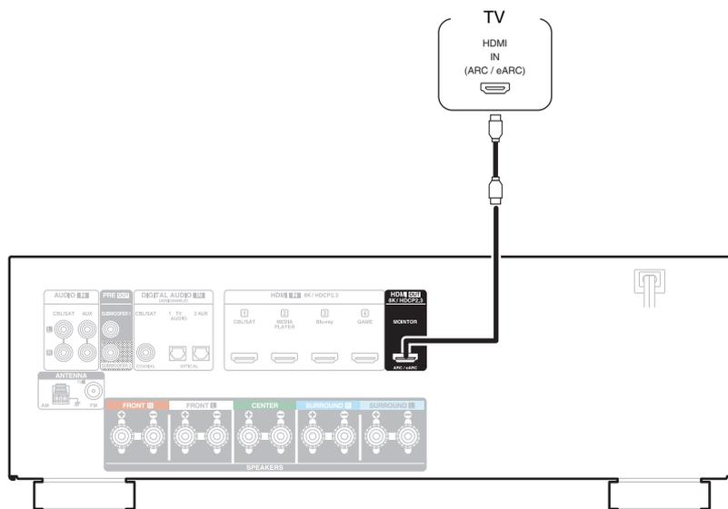
\* For 4K TVs we recommend using an HDMI cable labeled “High Speed” and “with Ethernet” .
