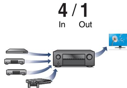
This unit is equipped with 4 HDMI inputs and 1 HDMI output enabling connection to various HDMI compatible devices such as Blu-ray Disc players, game consoles and HD video camcorders.
