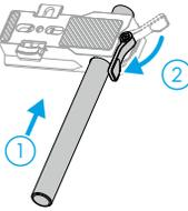
2. Attach the motor mount kit to the camera, and align the placement guide with the camera body before tightening the screw.
