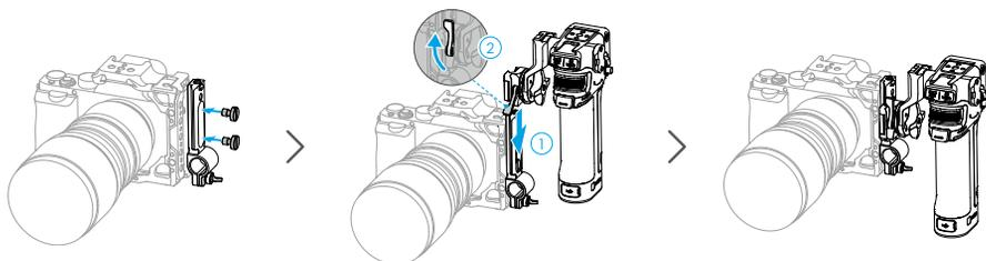
If the grip needs to be moved horizontally, attach the provided horizontal adapter slide rail before installing the grip. The direction of the NATO adapter mount can be adjusted, rotate the knob and pull the connector outward and rotate it counterclockwise, adjust the angle to install the grip to the horizontal adapter slide rail.
