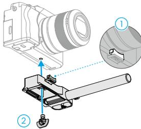
3. Attach the focus gear strip to the lens (if necessary). Attach the motor to the 15mm rod, and match the motor gear with the focus ring of the lens or the focus gear strip and tighten the clamp on the motor.
