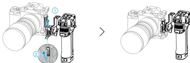
If the camera cage is not equipped with a slide rail, attach the provided rod adapter slide rail to the camera cage, and then insert the grip to the slide rail and lock the lever on the grip.
