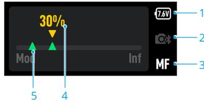
1. Displays the current battery voltage.
