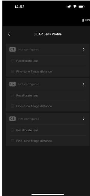
3. Tap Next to enter the focus ring calibration page, slide the focus ring to  $\infty$ , and then tap Confirm to start lens calibration. The lens profile will be saved after calibration is completed.
