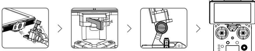
Ensure that Part B is unlocked. Install Part B into Part A.
