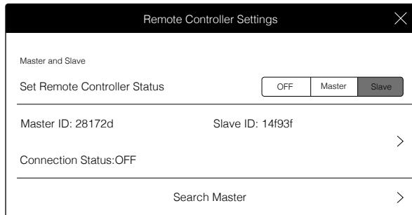
3. Select the Master remote controller from the Master list and input the password to connect.
