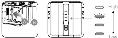
**⚠** Only use battery slot B when using one battery to supply power.
