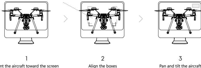
**⚠ DO NOT power off or unplug the USB cable after calibration. Wait for data calculation.**
