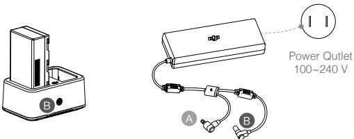
Using the WCH2 Charging Hub, charging time is approximately 1 hour and 11 min (one battery).
