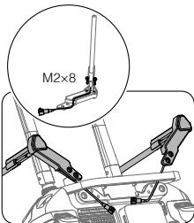
Thread the Datalink Pro antennas through the clips. Make sure that the lines of the antennas lie in the grooves of the mounting board where the clips attach to prevent the antennas from being damaged.
