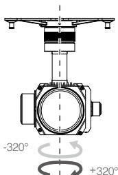
The right dial controls the gimbal pan. Turn the dial to the right, and the gimbal will shift clockwise. Turn the dial to the left, and the gimbal will shift counter clockwise. The camera will remain in its current position when the dial is static.
