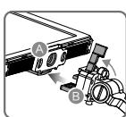
Ensure that Part B is unlocked. Connect Part B to Part A.
