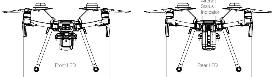
The Front LEDs show the orientation of the aircraft. Front LEDs glow solid red when the aircraft is turned on to indicate the front (or nose) of the aircraft. Front and rear LEDs can be turned off in the DJI GO 4 app. The Aircraft Status Indicators communicate the system status of the flight controller. Refer to the table below for more information about the Aircraft Status Indicators.
