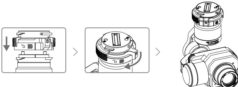
2. Then mount the Zenmuse XT onto the aircraft by securing the gimbal adapter.
