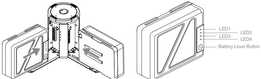
⚠ • Always align the grooves on the Intelligent Flight Battery with the battery slot tracks.
