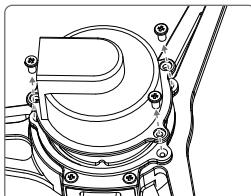
3. Disconnect the gimbal signal control cable and gimbal video coaxial cable from the single downward gimbal connector.
