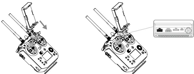
Unlock the Mounting Bracket and mount the Mobile Device Holder.
