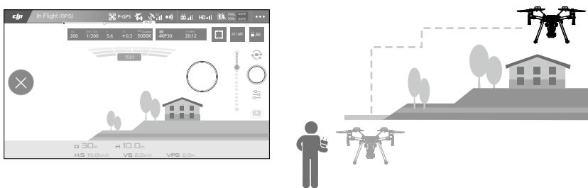
The aircraft automatically adjusts its speed when it senses an obstacle in front, or if it flies too close to the ground. The DJI GO 4 app will show a prompt if the aircraft flies over an obstacle or to the left or right of the obstacle. However, this feature should not be relied upon for navigation between obstacles. Failsafe procedures will override TapFly. If the GPS signal weakens, the aircraft will exit autonomous flight and return to home.
