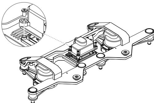
5. Connect the gimbal signal control cable and gimbal video coaxial cable to the dual downward gimbal connector accordingly. Tighten the spring pad with screws to secure the gimbal video coaxial cable.
