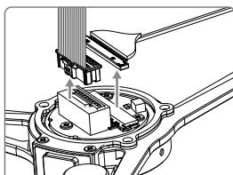
4. Remove the four screws on the top of the dual downward gimbal connector.
