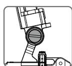
Use a coin to adjust the tightness of the tilt axis.
