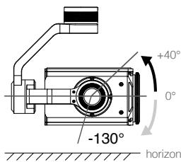
The left dial controls the gimbal pitch. Turn the dial to the right, and the gimbal will shift to point upwards. Turn the dial to the left, and the gimbal will shift to point downwards. The camera will remain in its current position when the dial is static.
