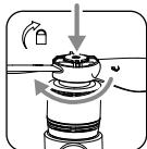
Press the propeller down onto the mounting plate and rotate in the lock direction until secure.
