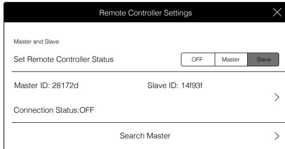
⚠ When in Slave, the remote controller cannot link to the aircraft nor control aircraft orientation. Select Master in DJI GO 4 if you wish to connect and control the aircraft with the remote controller.
