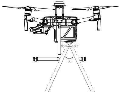
Infrared Sensing System detection range is depicted below.
