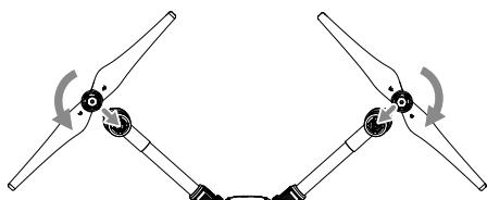
Check that the propellers are secure before each flight.
