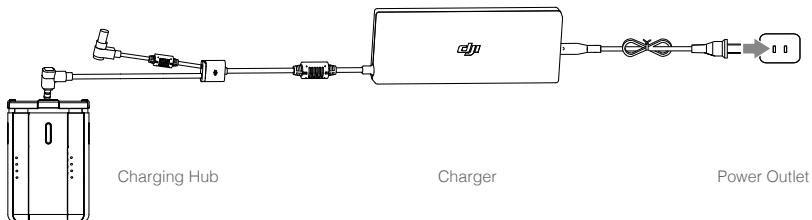
\* It will take approximately 1.5 hours to fully charge the TB50-M200 Intelligent Flight Battery, and 3 hours for the remote controller. It will take a longer time to charge the Intelligent Flight Battery and remote controller together.
