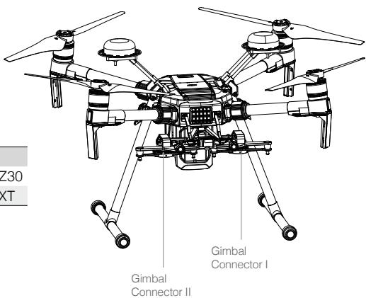
Note that the gimbal connector II can be mounted with Zenmuse XT and Z30 only, and gimbal connector I and gimbal connector II cannot be mounted with two same Zenmuse gimbals.
