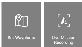
Waypoint flights can be planned in two ways: Set Waypoints or Live Mission Recording. Use Set Waypoints to create a route by adding and editing waypoints on the map. Use Live Mission Recording to create a route by adding waypoints when taking photos along the route.
