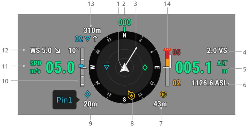
1. Aircraft: the attitude indicator will rotate as the aircraft changes its orientation.
