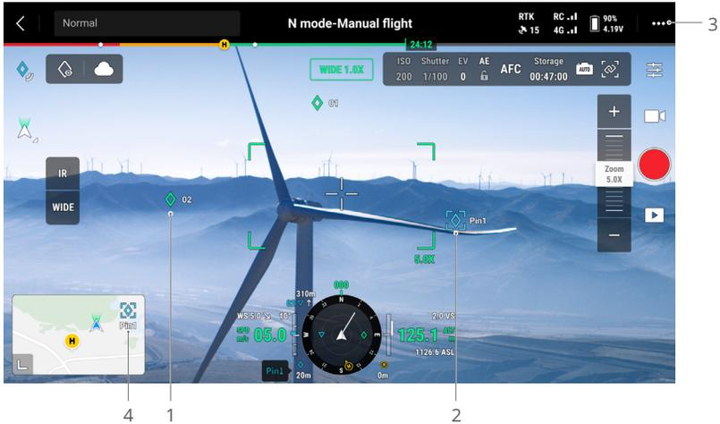
1. AR projection will be created for the PinPoint in the camera view. PinPoint size will be adjusted according to the distance between the aircraft and the PinPoint (big when near, small when far).
