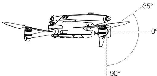
Use the gimbal dial on the remote controller to control the tilt of the camera. Alternatively, enter the camera view in DJI Pilot 2. Press the screen until a circle appears and drag the circle up and down to control the tilt of the camera.
