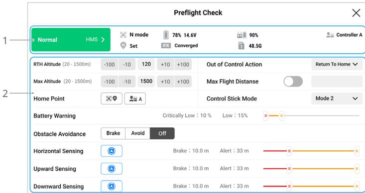
1. View the aircraft's health information, flight mode, intelligent flight battery level, remote controller battery level, home point status, RTK status, and camera microSD card storage information.
