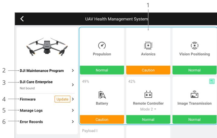
1. Error Diagnosis: for checking the current status of each aircraft module. Users can solve issues by following the corresponding prompted instructions.
