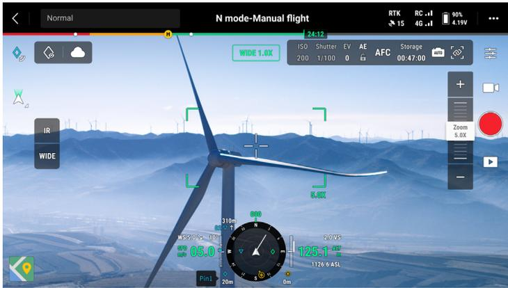
Zoom Frame: after switching to the wide mode as the main view, the field of view and camera zoom ratio will be displayed on the zoom frame.
