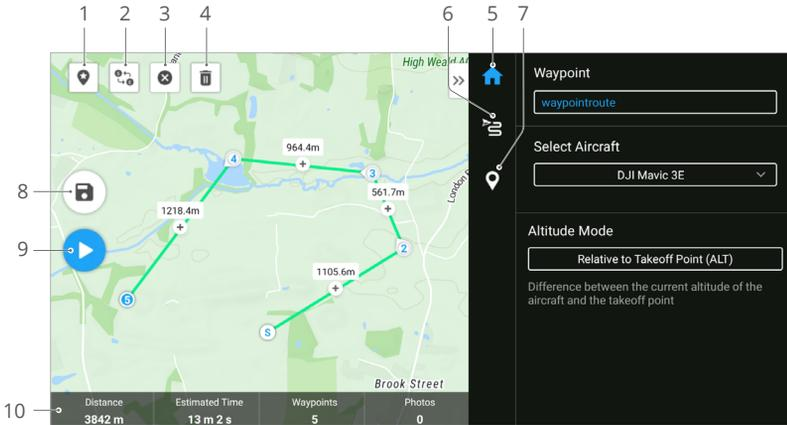
1. Point of Interest (POI): tap to enable the POI feature, and a POI will be displayed on the map. Drag to adjust its position. After a POI is added, the aircraft yaw can be set as facing the POI, so the aircraft nose always faces the POI during the task. Tap this icon again to disable the POI feature.
