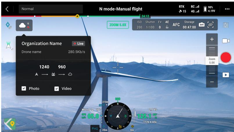
21. Flight Task Status: displays the progress of a flight task in the camera view. Tap the Pause/Resume button to pause or resume the task and tap the panel to view the flight task details.
