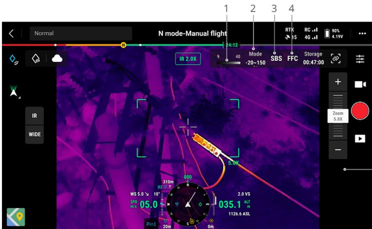
1. Palette: displays the highest and lowest temperature measurement values of the current view. Tap to choose between different infrared temperature measurement palettes or enable the isotherm to set temperature measurement intervals. Note that if the measured area exceeds the maximum or minimum temperature measurement values of the current view, the setting will not take effect.
