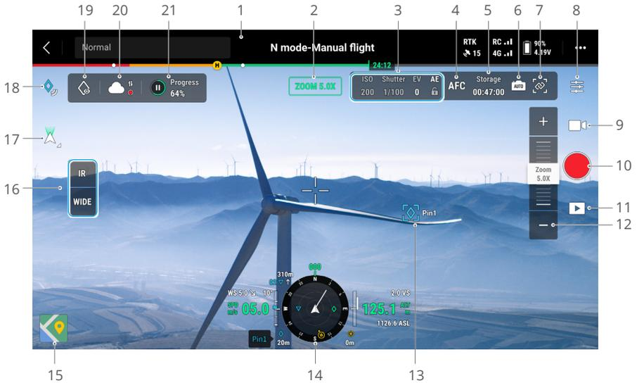
1. Top Bar: displays the aircraft status, flight mode, signal quality, etc. Refer to the Top Bar section for more details.
