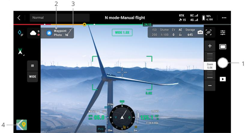
1. Control the gimbal, adjust the zoom scale, and aim at the target. Tap to capture photos or press the C1 button of the remote controller to add a waypoint. The number of waypoints and photos will be added accordingly.
