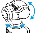
Follow is selected by default. In this mode, the pan and tilt axes follow the handle while the roll axis remains level. This mode is suitable for most scenarios, including vlogs and selfie videos.
