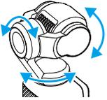
In this mode, the camera rotates freely and follows the handle movement. This mode is suitable for scenarios where the camera position is continuously rotating and there is less stability.
