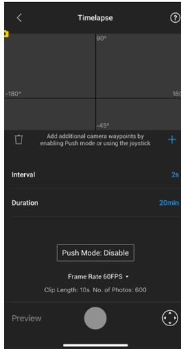
In Timelapse, the gimbal triggers the camera to capture still images with the set interval time and will automatically stop when completed. The duration for the Timelapse and the frame rate can be set so that the gimbal can calculate the exact number of images required.
