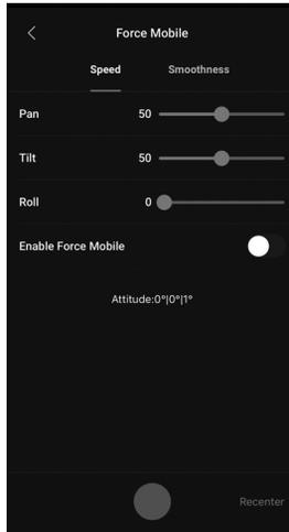
Force Mobile requires the phone holder and a mobile phone mounted on a tripod or handlebar vertically.
