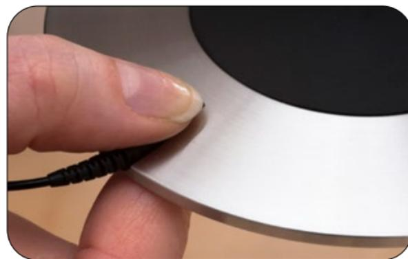
**The cable is connected to the microphone by turning the lock cap clockwise.**
