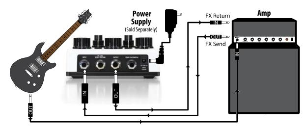
Use only unbalanced instrument cables for audio connections.
