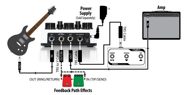
Use only unbalanced instrument cables for audio connections.
