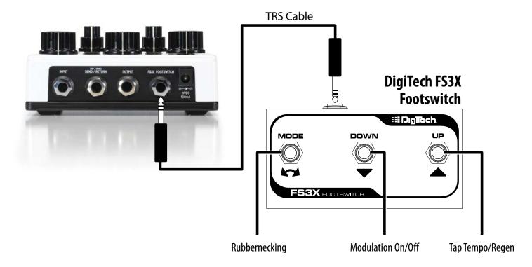
**NOTE:** For full functionality, connect the DigiTech FS3X Footswitch using a TRS cable. A TS cable can be used to control Tap Tempo and Regen when using a third party momentary footswitch (latching footswitches will not work). When using a third party momentary footswitch with a TS cable, it must first be connected to the Rubberneck before applying power to allow the Rubberneck to detect it and function correctly.
