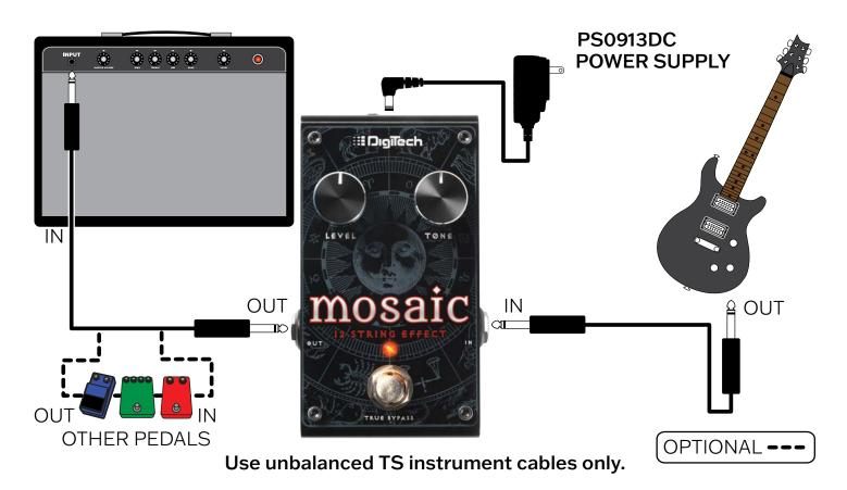
**NOTE:** The Mosaic should be the first pedal in your effects chain. Placing any effect in front of it may impact its pitch shifting performance.
