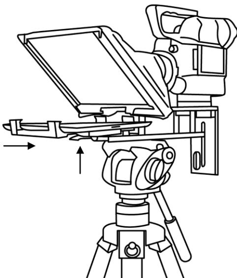
13. Put the configured tablet into the mounting bracket and ensure it is held securely by adjusting the size of the bracket holders for a snug fit and locking them in place. Use the locking lever on the bottom of **item E**.
