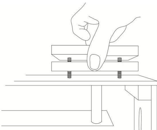
When using this TP-300 Prompter Kit you may need to use one or both riser blocks to raise the camera up so that the camera lens is positioned vertically as near to the middle of the 60/40 Glass as possible.
