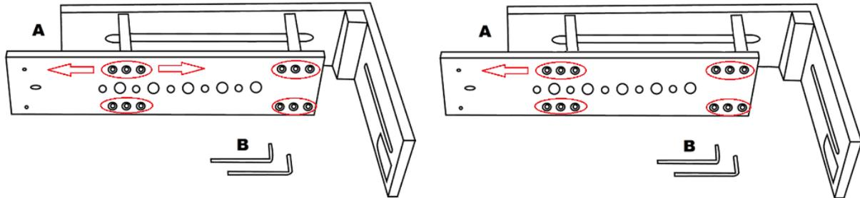
1. First carefully dismantle the current TP-300 set up to remove the prompter frame (Item A).
