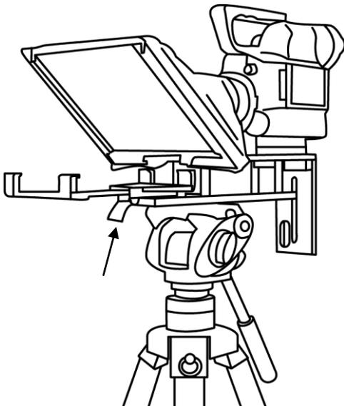
11. Fit the adjustable mounting bracket, **item E**, to the Prompter Frame just below the Glass Frame using the mounting bracket screw, **item D**, and the recess in the Prompter Frame.
