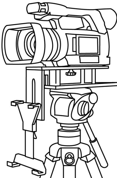
3. Fit the camera riser screw, **item O**, from below the prompter frame's long top slot. Marry the camera's base plate screw hole with Camera riser screw and secure the camera to the frame. Adjust position of the camera so the camera lens is at the edge of the prompter frame.
