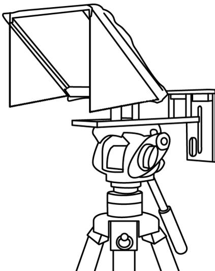
6. At this point decide if you want to fit the optional side curtains. Generally the side curtains should only be fitted when working in direct sunlight.
