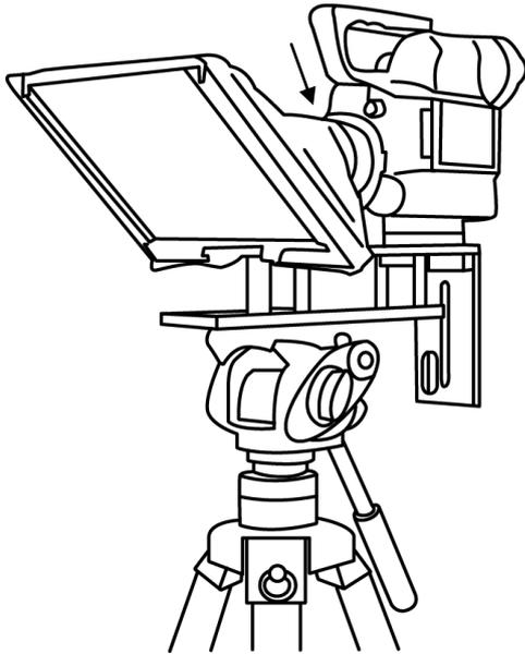
10. Pull the draw cord to secure the black camera Snood / Hood around the camera lens and to shut out light from camera side.
