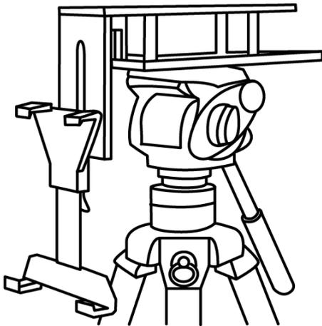
2. Use the mounting bracket screw, **item D**, to secure the mounting bracket for the tablet computer to the front of the Prompter frame's vertical plate.
