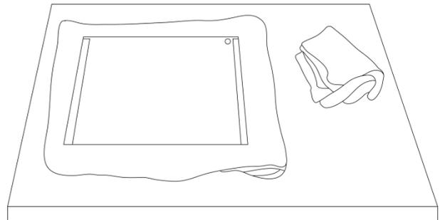
Once finished re-install the glass back into the prompter hood, again using the cloth covered edges only. **Ensure the green circle sticker on the glass is facing you** and the red circle sticker is facing the camera lens. Reseat/secure the camera hood if necessary.
