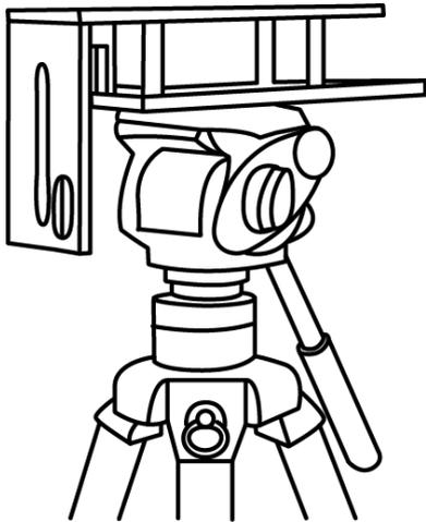
1. Attach/screw the tripod camera quick release plate to the screw holes on the base of the prompter frame, **item A**. If necessary use the adaptor screw, **item C**. Slide and secure the tripod plate, with prompter frame on top, onto the head of tripod. Ensure the vertical plate of the prompter frame is facing toward the on screen talent / commentator.
