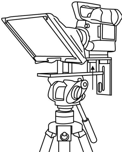
8. Fit the camera riser screw, **item O**, with washer from below the top slot, through the riser blocks centre hole and into the camera base, so the camera is secure with prompter block(s) and frame.
