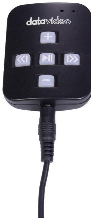
**NOTE:** When using this remote in wired mode the **DV Prompter Plus app** should also be set to **Wired – WR-500** in the **Remote menu option**.
