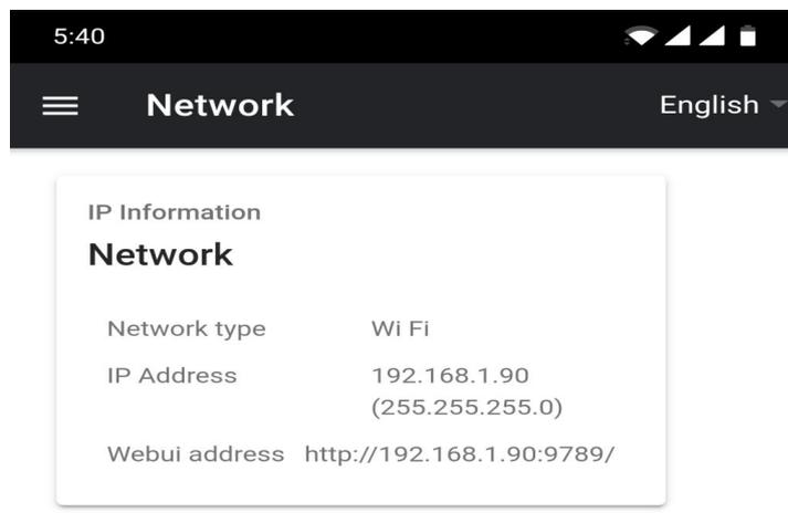
2. Open the settings menu on the slave device, enable slave mode and enter the IP address of the master.
