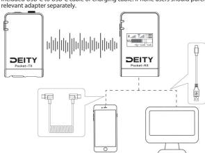
\* Pocket Wireless works out of the box with Cameras, Recorders, Smart-phones, Laptops, and Tablets that feature "Plug-in-Power" via the USB-C to USB-C cable or charging cable.
