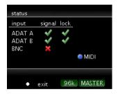
The *status screen* is a useful help when configuring the A16 AE, giving an overview of the digital inputs. To activate it, press **MENU** and then select *status*. The screen shows for every digital input, whether it receives a valid signal (*signal*) and whether this signal's sampling rate is correct (*lock*). Only if both conditions are met, the A16 AE will use the signal.
