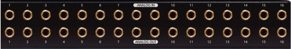
All analog inputs and output can be found on in balanced ¼" (6.3mm) TRS jacks, and can be set independently to a level/sensitivity between -8dBu and +20dBu. All inputs and outputs are fully balanced.
