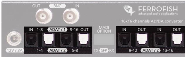
Each ADAT interface can transfer eight channels at SMUX/1. When using SMUX/2 the channel count reduces to 4. Since the PULSE16 is equipped with four ADAT interface In/Out pairs, transfer of all analog 16 input and 16 output channels is still possible.
