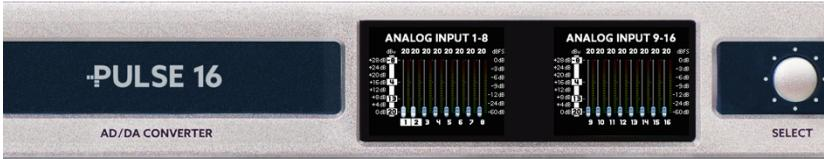
The number above the fader shows the maximum level in dBu, which the input can handle. When the fader is set to “20” like in the picture above the input can handle an maximum input level of +20dBu. Avoid exceeding this maximum level to prevent digital clipping.
