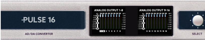
The dB scale on the right side shows the resolution of the metering levels. This scale does not show the level value of the fader!
