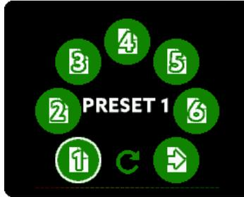
After selecting the desired preset by using the SELECT pot and MENU to load it a second screen appears. This screen lets you choose what should be loaded: The GAINS of the analog inputs, the LEVELS of the analog outputs, the routing – or all three items.
