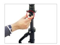
Mount the gimbal support on the baby pin stand and secure it with the help of the knob, as shown in the image.
