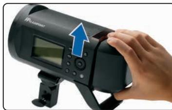
2. Then, slide the Battery Release to the right while lifting the battery pack upward, out of the connection.
