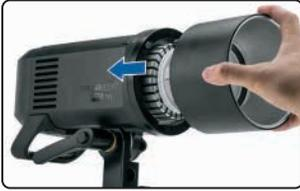
1. Press down the Reflector/Modifier Lock Release lever.
