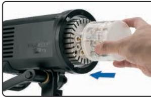
2. Align the 4 Flashtube pins to match the protruding rings in the Tube Socket [4] surrounding the LED Modeling Lamp [3] on the XPLOR body. Push the flash tube in firmly until it is securely seated into the socket. The flashtube can be handled without protective gloves as the outer glass shields the actual flashtube.
