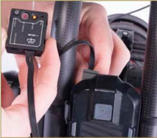
2. Power up the MōVI Controller and set the channel on MōVI Controller to match the channel on the MōVI RX.
