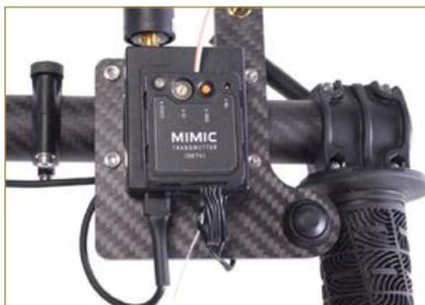
4. Turn on the MōVI Pro and make sure the MIMIC Beta TX and Freely RX status LED are illuminated, indicating both have power.
