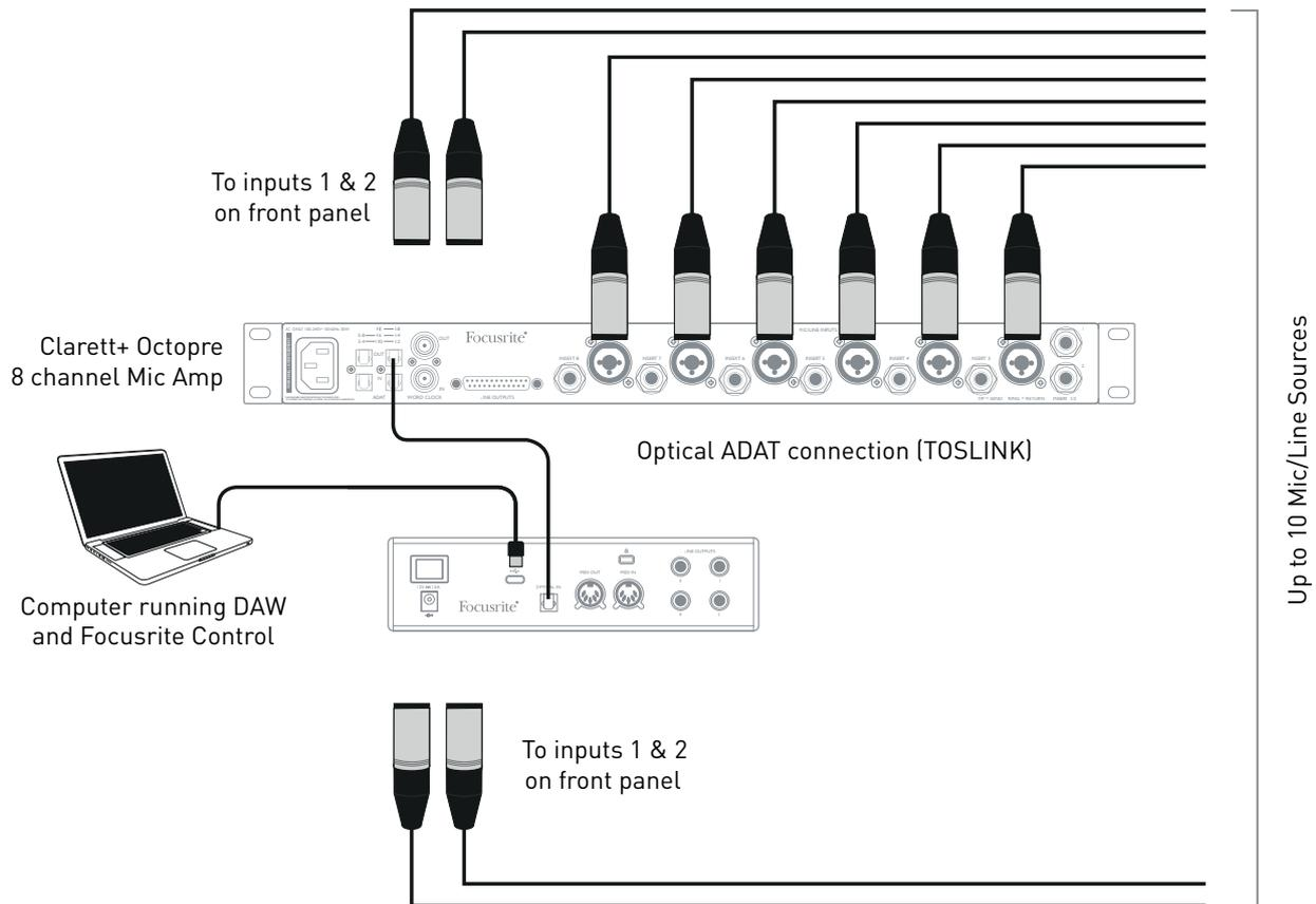
The Clarett+ v’s **OPTICAL OUT** port is connected to the Clarett+ 2Pre’s **OPTICAL IN** port with a single TOSLINK optical cable. The two devices must be synchronised to ensure audio passes cleanly, without clicks and pops. To do this in **Focusrite Control** go to **Device Settings** and set the **clock Source** to **ADAT**. Both devices must be set to the same sample rate.
