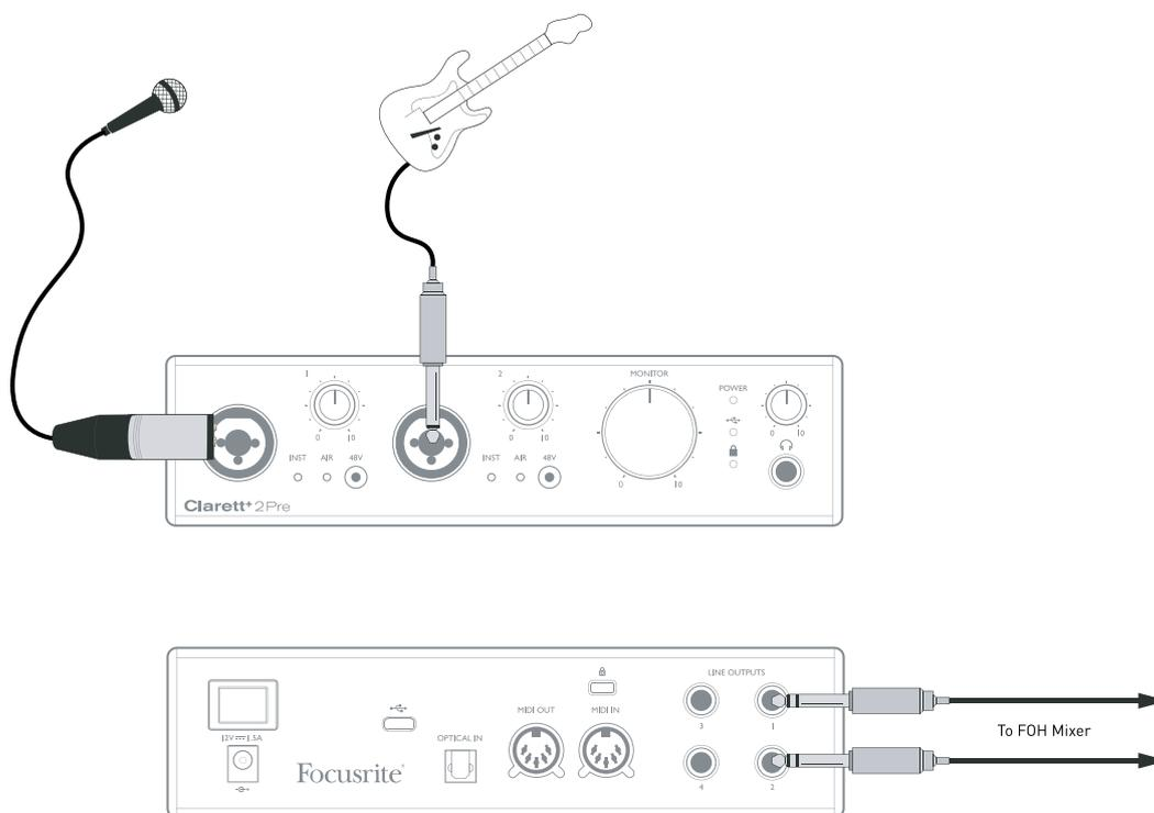
In the example illustrated, a mic and a guitar are connected to the Clarett+ 2Pre's inputs; Outputs 1 and 2 go to the main PA system. The performer can adjust the mic and guitar volume separately from the front panel.
