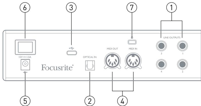
1. **LINE OUTPUTS 1 to 4** – four balanced analogue line outputs on ¼” jack sockets; use TRS jacks for a balanced connection or TS jacks for unbalanced. Line Outputs **1** and **2** will generally be used for driving the main L and R speakers of your monitoring system, while Outputs **3** and **4** can be used for connecting additional line level equipment (e.g., outboard FX processors). Signals routed to all the outputs may be defined in **Focusrite Control**.
