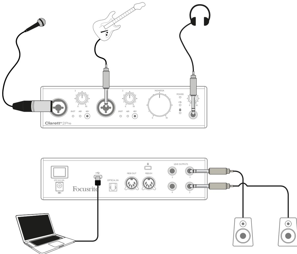
This setup illustrates a typical configuration for multitrack recording with DAW software on your computer.
