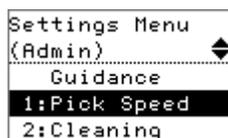
To switch between the menus, press down both the [ $\Delta$ ] and [ $\nabla$ ] buttons at the same time for three seconds or longer while the [Settings Menu] screen is displayed.
