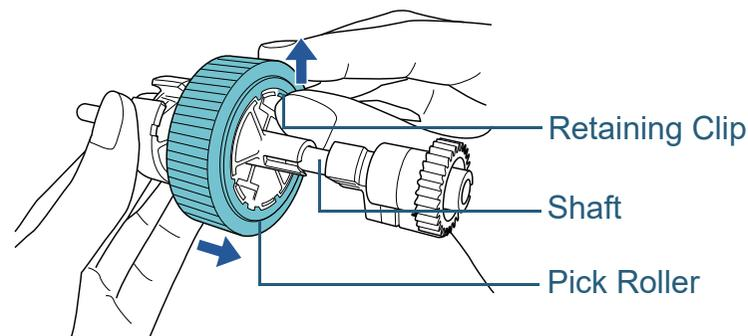
**6** Attach the two new pick rollers on the shaft one at a time.
