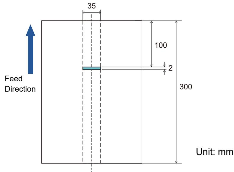
Since the detection range (length) is less than 5 mm, multifeeds cannot be detected accurately.
