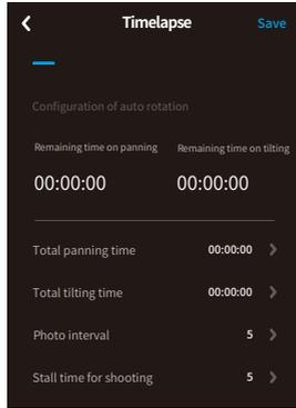
**Method 2** Set the Motion-timelapse mode parameters by entering the "Motion Timelapse" interface through the touch screen.
