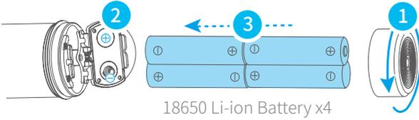
⚠ Please properly check the cathode and anode of battery before put the battery on, the gimbal can't be turned on with wrong battery mounted.
