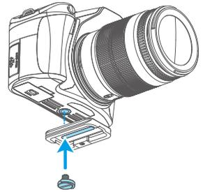
(3) Insert the secondary quick release plate tiltly and press down. The secondary quick release plate safety lock automatically locks and be firmly tighten.
