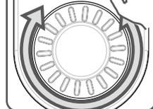
**4. Power option:** press the GR/CH button and power the light on to enter power option mode. Turn the brightness select dial to choose power from 300, 250 and 200. The power is 300W by default. Exit from this mode automatically without operation for 5 seconds.
