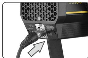
2. Plug the output end of adapter's connect cord into controller's power input end.
