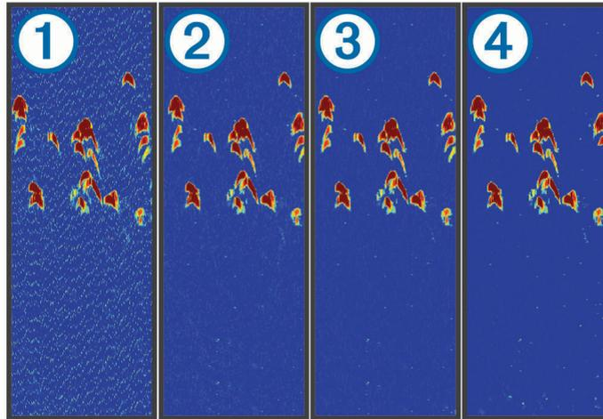
When you adjust the interference setting from off ① through low ②, medium ③, and high ④, noise is gradually removed, but there is little effect on the strong target returns. You should use the lowest interference setting that achieves the desired improvement to remove interference from the screen. Correcting installation issues that cause noise is the best way to eliminate interference.
