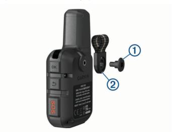
2 Secure the spine mount adapter 1 over the back of the device using the long screw 2 included with the device
