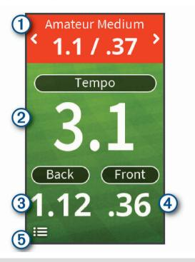
Displays the tempo timing (backswing to downswing time ratio). Changes the tempo timing when selected.
