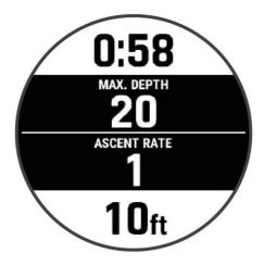
**In-dive screen**: Displays the information about the current dive, including the elapsed time, current and maximum depth, and rate ascent or descent. You can edit the data screen layout and data fields (*Customizing the Data Screens*, page 116).
