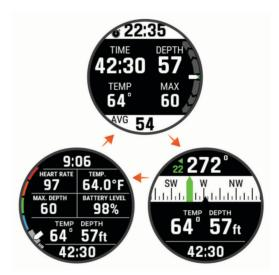
**Dive stopwatch**: Displays the bottom time stopwatch; current, maximum, and average depth; and rate of ascent or decent (*Using the Gauge Dive Stopwatch*, page 19).
