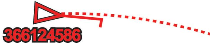
When course over ground and heading information are provided by an activated AIS target, but rate of turn information is not provided, the projected course of the target is calculated based on the course over ground information.
