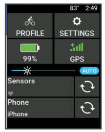
The status widget appears. A flashing icon means the device is searching for a signal. A solid icon means the signal was found or the sensor is connected. You can select any icon to change the settings.
