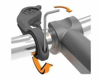
6 Open the locking ring ③.NOTE: The locking ring is in the open position when the red line is visible on the side of the mount.
