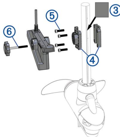
**NOTE:** The rubber liner is not needed when installing the transducer on a trolling motor with a shaft diameter that is larger than 25 mm (1 in.), such as the Garmin Force trolling motor.
