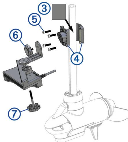
**NOTE:** The rubber liner is not needed when installing the transducer on a trolling motor with a shaft diameter that is larger than 25 mm (1 in.), such as the Garmin Force® trolling motor.
