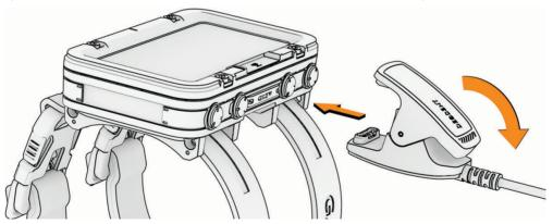
**3** Plug the USB cable into a USB charging port.
