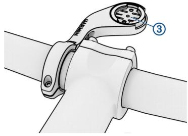
7 Press down slightly and turn the Edge bike computer clockwise until it locks into place.
