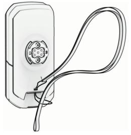
2 Thread the other end of the tether through the loop, and pull it tight.
