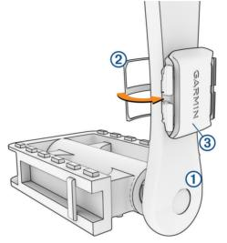
4 Rotate the crank arm to check for clearance.
