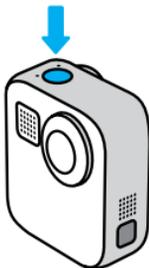
2. Press the Shutter button
