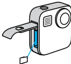
You can eject the card by pressing it into the slot with your fingernail.
