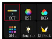
**CCT MODE** : White light mode with adjustable light intensity and color temperature.
