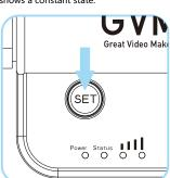
3 When the Status indicator start to fast blinking, it indicates that the connection with the transmitter is in progress. After successful  $% \left\{ 1,2,...,n\right\}$ connection, the Status indicator turns to constant state and the signal indicator shows the signal strength.
