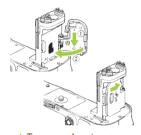
To prevent loss, insert the battery chamber cover into the camera battery chamber cover storage slot on grip.
