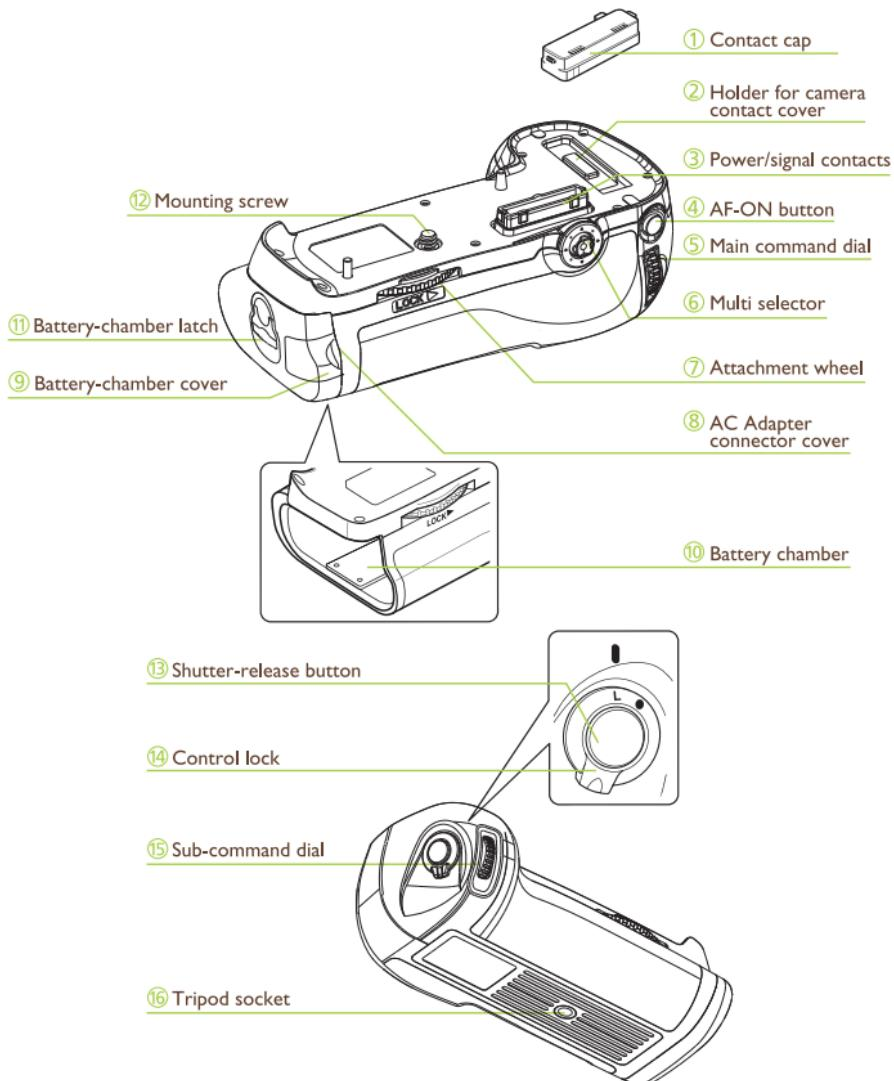
The MB-D12 Shutter-Release Button, Multi Selector, Command Dials, and AF-ON Button.
