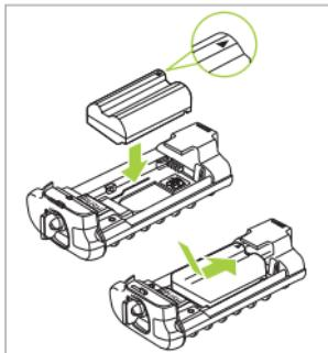
1. Ensure that the power is turned off on the camera and the Control Lock on the grip is in the "L" position. Turn the battery-chamber latch counter-clockwise to open the battery chamber door.
