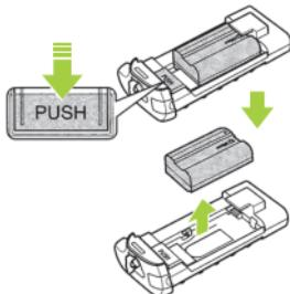
The procedure for removing the EP-5B power connector is the same as that for the EN-EL15.
