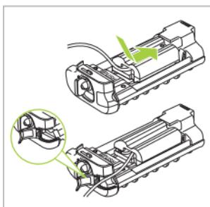
4. For AA Batteries: Place eight AA batteries of the same type in the AA battery holder, while ensuring that they are in the correct orientation. Mixing old and new batteries may cause accident.
