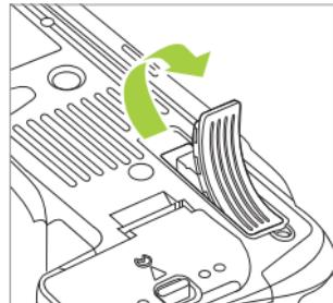
1. Please turn off the camera and ensure that the Control Lock on the grip is in the "L" position before attaching.
