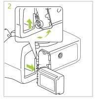
Open the camera's battery chamber cover and remove the battery.
