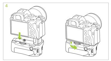
4. Insert the grip's electrical control bar in the camera's open battery chamber. Slide the grip into the chamber until the camera base meets the grip and carefully align the grip attachment screw with the camera's tripod socket. Turn the attachment wheel in the direction of the arrow to securely join camera and grip.
