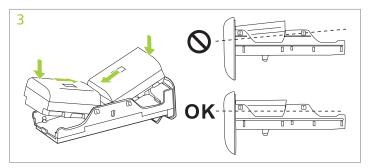
3. Place each NP-FZ100 battery module in its space, carefully aligning the cells to lay flat in the channel to assure firm contact in the tray. One cell can be used. The tray has space for two cells.
