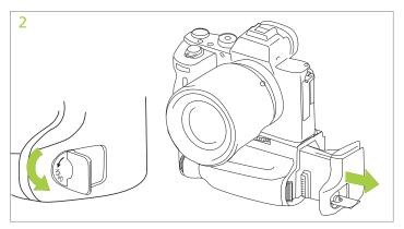
Open the battery chamber by turning the latch counterclockwise. Slide the battery tray from the grip body.
