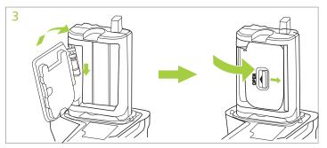
Attach the chamber cover onto the battery compartment cover storage (12) for safe keeping on the grip.
