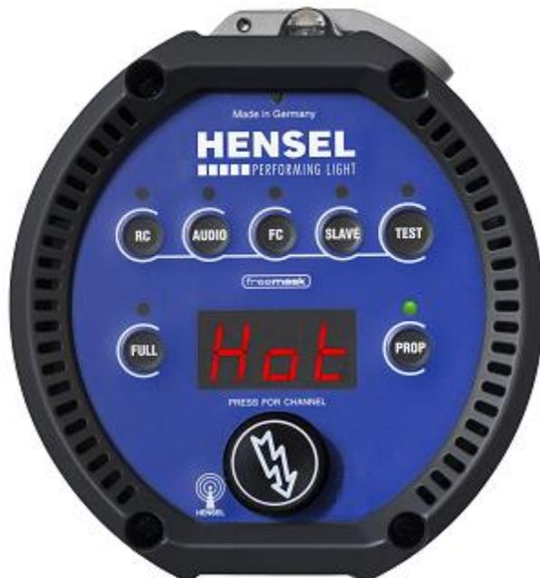
In case of this problem, the modeling light shuts off, the fan blows at full speed and the unit stops flashing.
