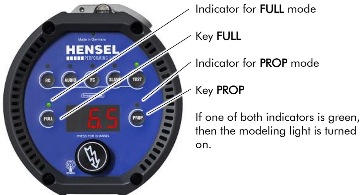
If none of both indicators is green, press the key **FULL**. The indicator above the button turns green and the modeling light is turned to maximum brightness.
