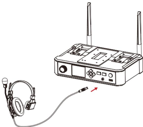
1. Plug the headset into the 0B10 headset interface on the hub and rotate the nut clockwise to secure the headset.
