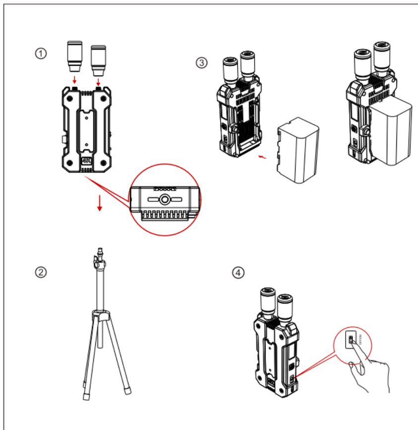
① **Install the antenna shown in the picture.**
