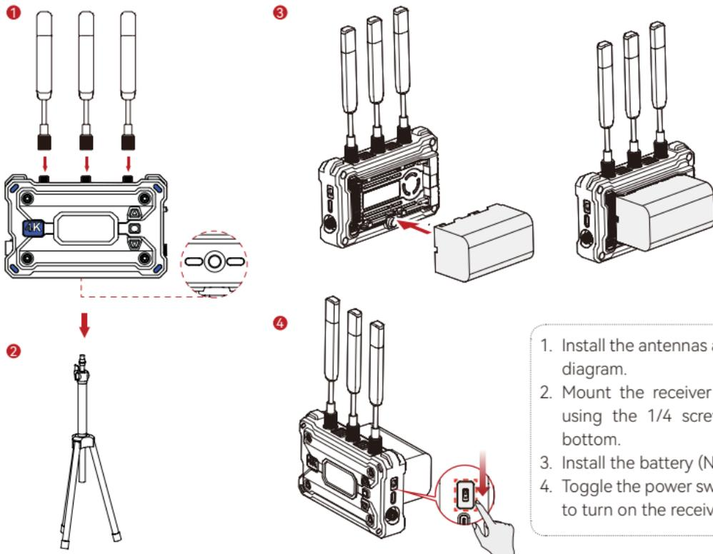
1. Install the antennas as shown in the diagram.
