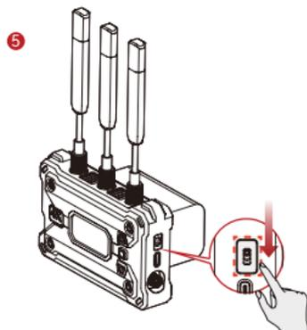
1. Install the antennas as shown in the diagram.
