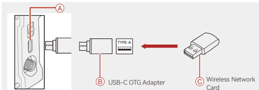
1. Connect the wireless network card to the transmitter using the USB-C OTG Adapter.
