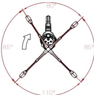
Microphone mute range when moving the microphone boom upward clockwise
