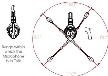
Microphone mute range when moving the microphone boom downward anti-clockwise
