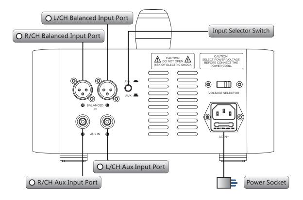
\* Make sure the power supply switch corresponds to local mains voltage before connecting to power socket.
