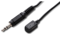
Figure 13 – IR Emitter Cable CIR-EMT (Emitter has adhesive backing) Pin out: Tip=Anode, Ring=Cathode, Sleeve=Not Connected
