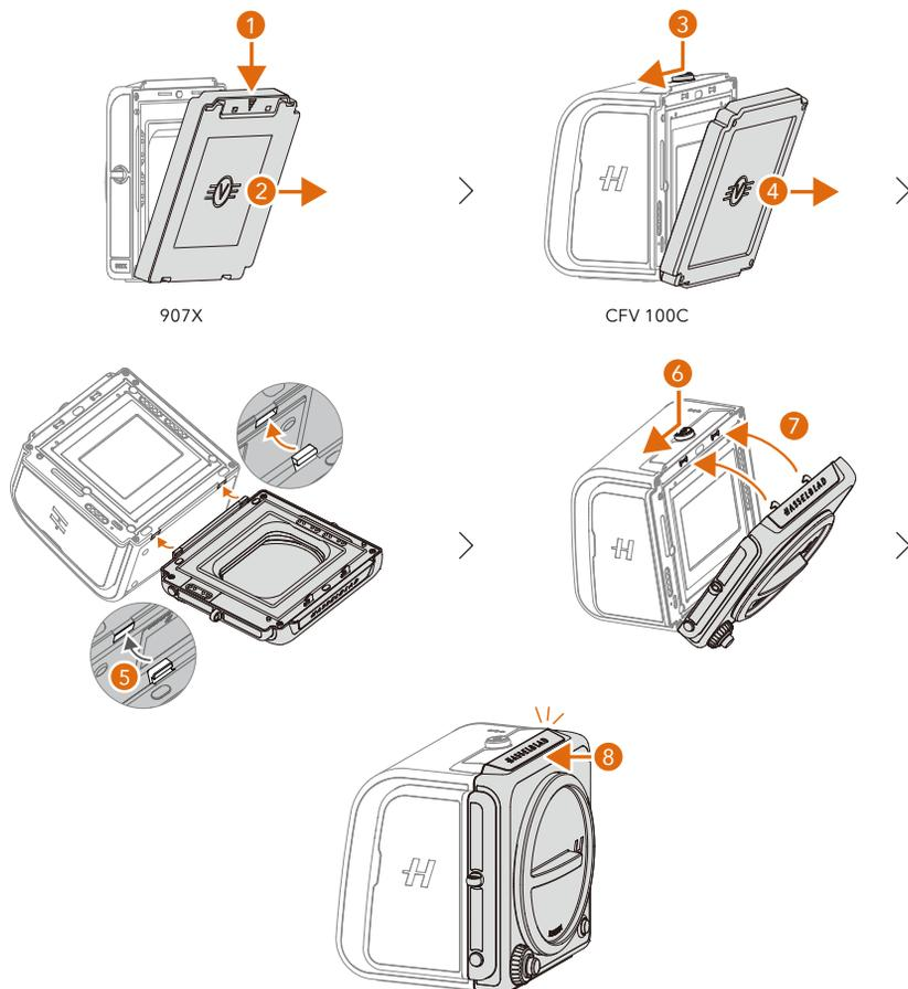
1. Remove the rear protective cover of the 907X camera body by pressing on the top of the cover (1) and then swinging it backwards (2).
