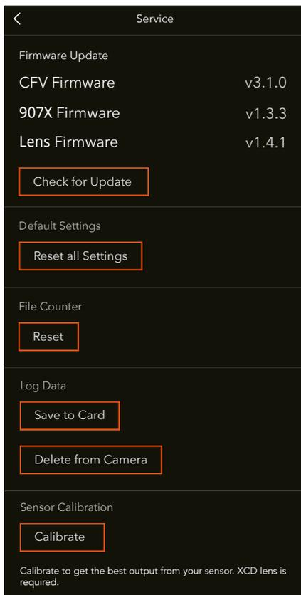
6. The camera will update firmware automatically. It will take several minutes for the update to complete. DO NOT power off the camera or remove the memory card if in use during an update.
