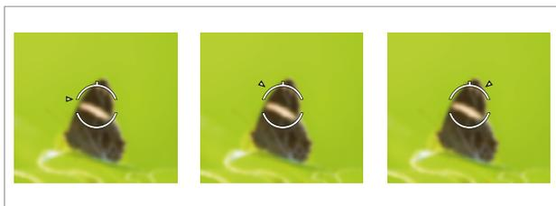
White triangle: The focus is close to the subject. Users can rotate the focus ring to focus. Rotate the focus ring clockwise when the triangle is located on the left of the focus indicator. Rotate the focus ring counterclockwise when the triangle is located on the right.
