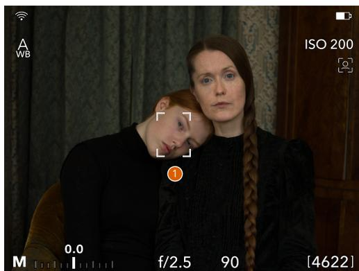
1. When a face is detected, the detection result will be displayed in the grey frame (1).
