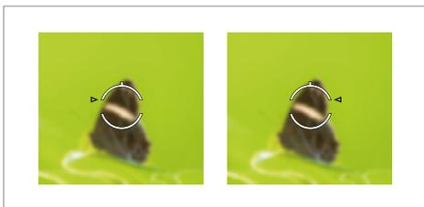
Grey triangle: The focus is too far from the subject. Users can try to rotate the focus ring clockwise or counterclockwise to make the triangle turn white.
