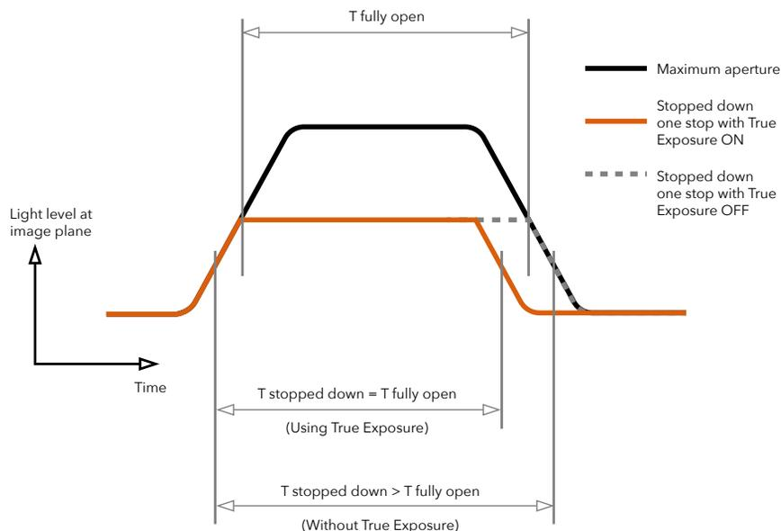
True Exposure is an XCD and HC/HCD lens function that allows the shutter speed to remain unaffected when stopping down. This effect is perhaps not so commonly understood as it is restricted specifically to integral lens shutters as opposed to focal plane shutters.
