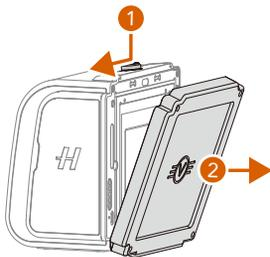
1. Press and hold the lock button on the top of the digital back and push it to the direction as shown in the figure (1) and remove the protective cover (2).
