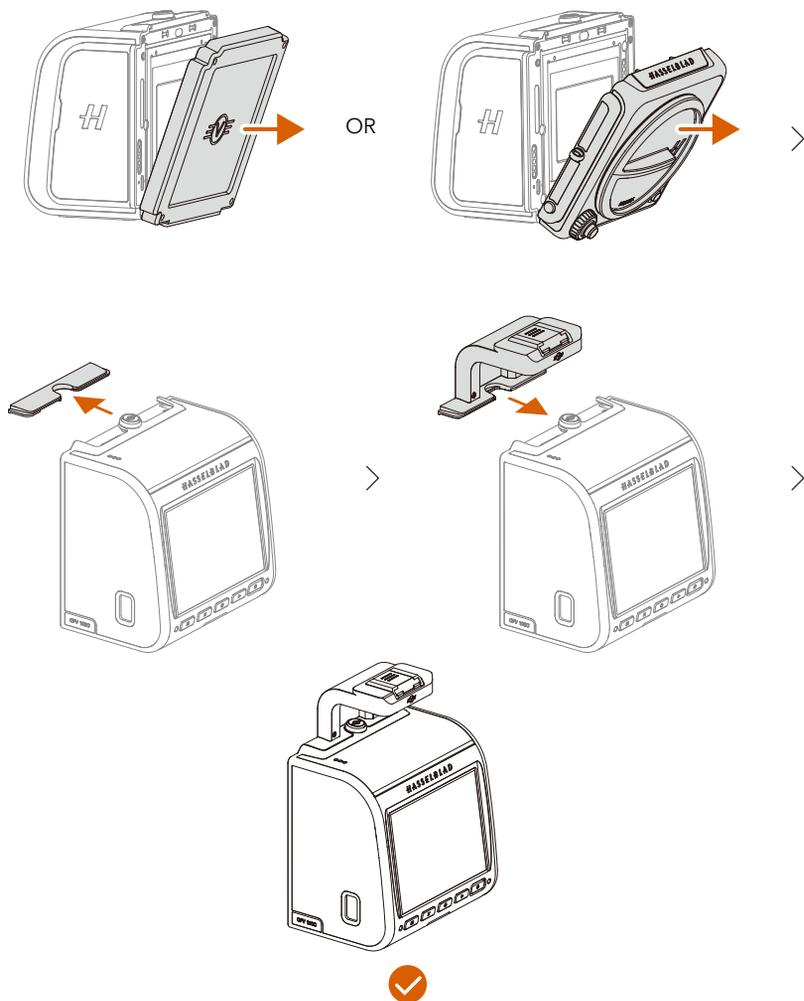
1. Detach the digital back from the connected device.
