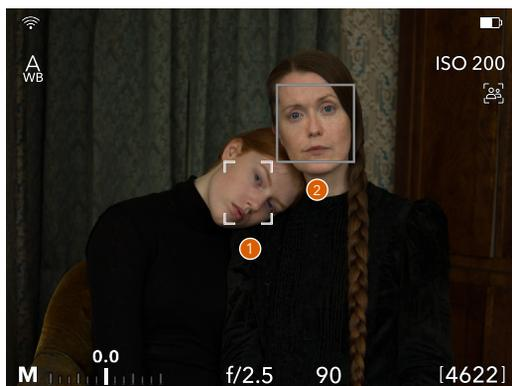
1. Multiple faces are detected. Only one of the detection results will display the grey frame (1), indicating that it will be focused on after pressing the shutter release button. Other detection results will display the grey frame (2).
