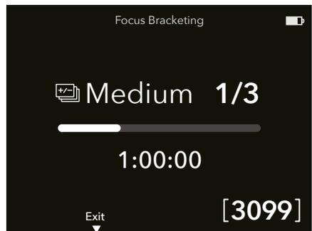
**Step Size:** The step of the focus position between frames. Refer to the following section for more information.
