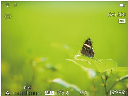
The focus indicator can indicate the relationship between the focus and subject and show the direction to rotate the focus ring.
